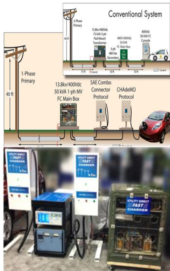
Figure 11: Utility Direct Fast Charger (UDFC)
